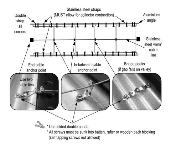
For tile roofs this mid panel cable is an easy retro-fit and we recommend its installation, see new manual under Wind Proofing section.
