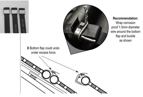
If you have installed these straps, we strongly recommend applying the wire fixings as shown. However before carrying out this fix please check that the straps are not too tight.
