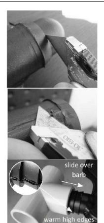
**BEFORE CUTTING - put aside two collectors per row with <u>undamaged</u> <b>end caps.** For all remaining collectors cut the single end cap off using a sharp blade or hacksaw.
